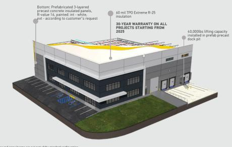
\*Cranes and crane beams are not part of the standard configuration
