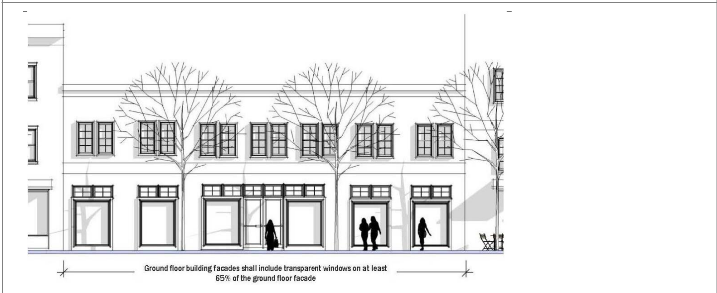
FIGURE 536-5 GROUND FLOOR WINDOWS
