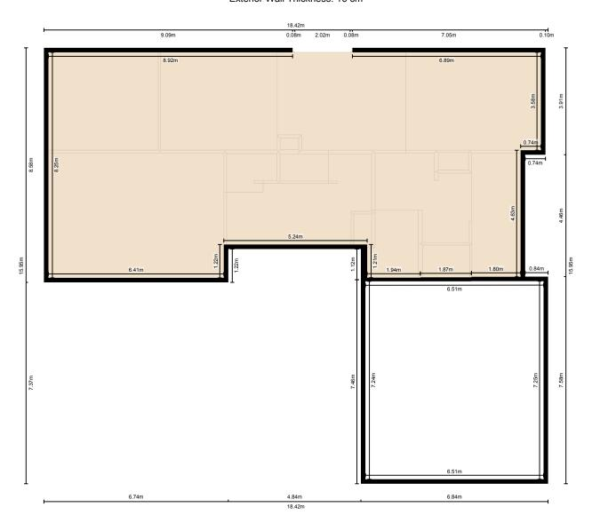
Measurement Diagram for: 2nd Floor Exterior Wall Thickness: 16 cm
