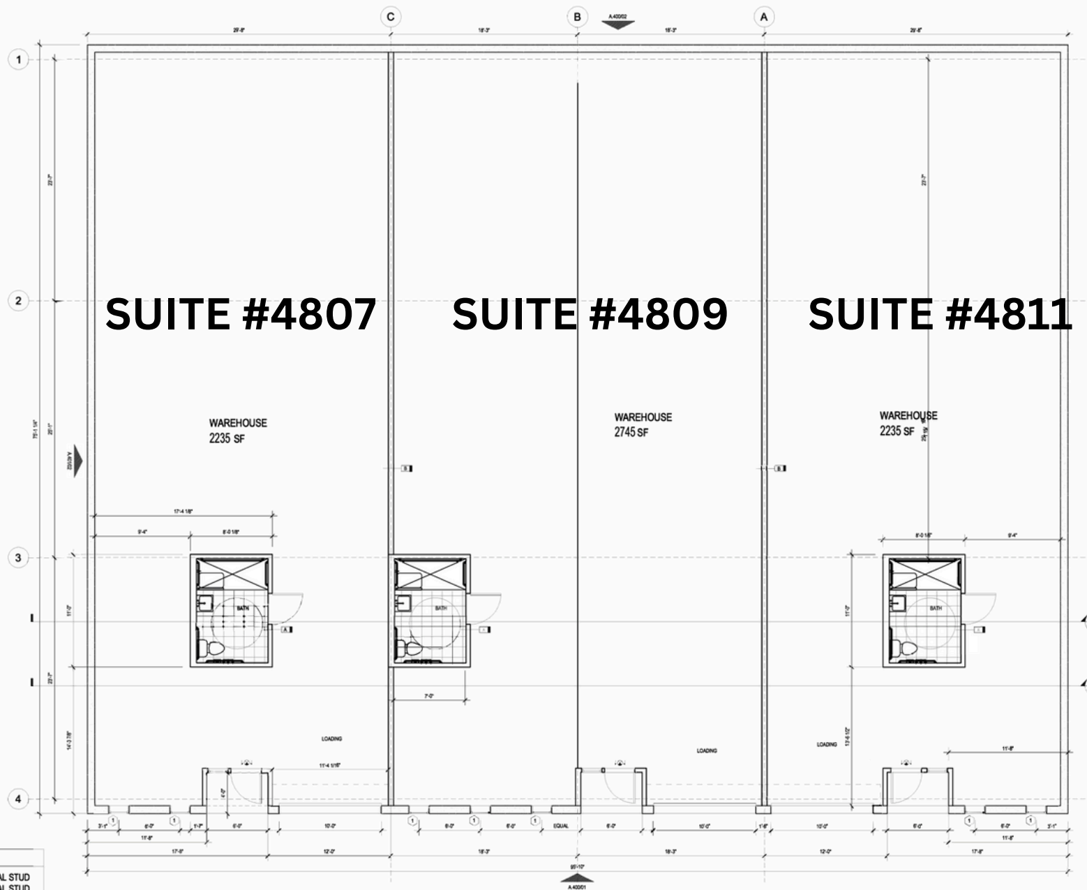
01 4807 NORMA - NEW FLOOR PLAN SCALE: 1/4" = 1'-0"
