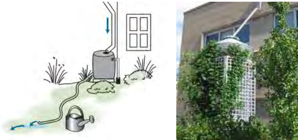
Examples of rainwater harvesting (Source: United States Environmental Protection Agency)
