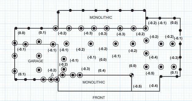
INSTALLED 58 TOTAL PILINGS (23 EXTERIOR, 35 BREAKOUTS).
