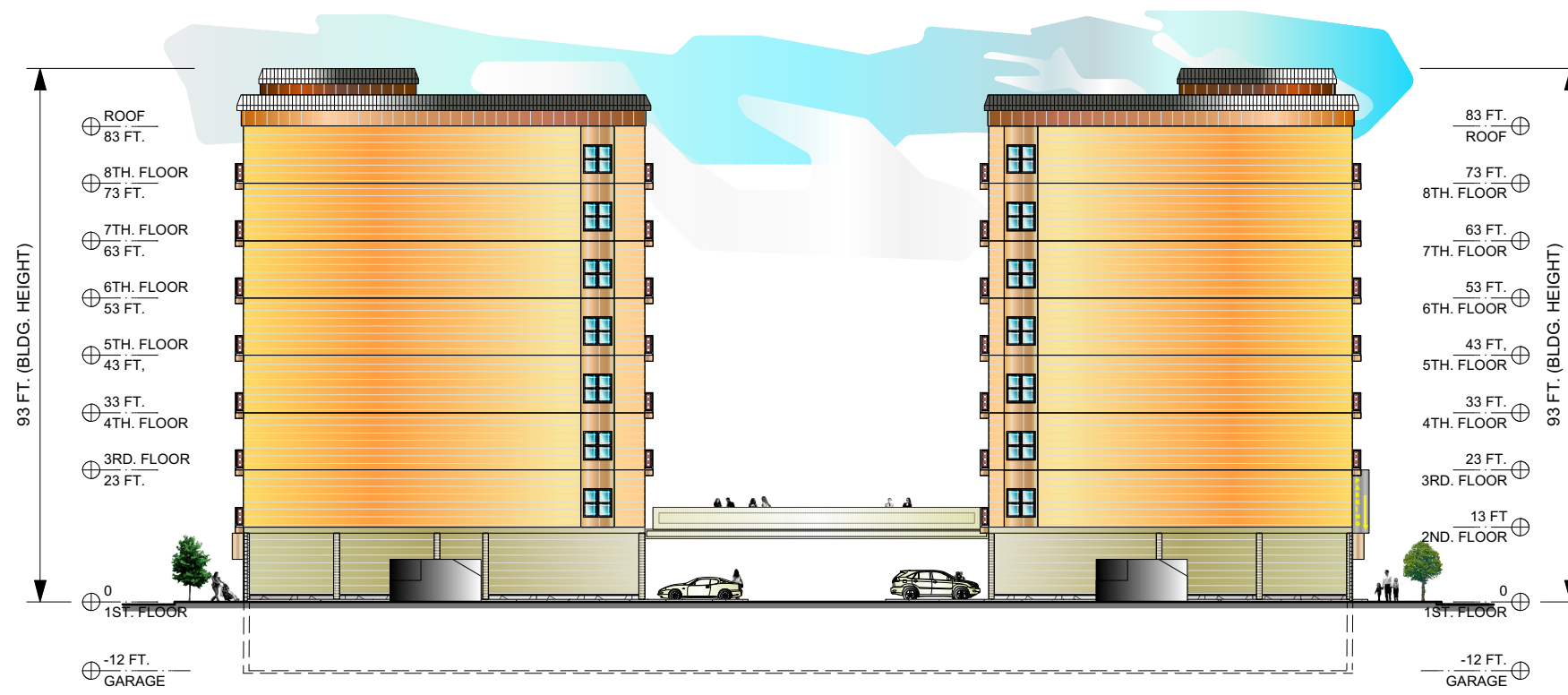
LEFT SIDE ELEVATION (SERVICE AREA) Scale: 1" = 30 ft
