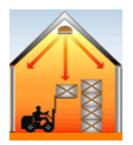
Low Intensity Infrared Heating System: Radiant heat minimizes roof heat losses by directing heat downwards to the area that requires heating. Radiant heating heats in the same manner that the sun warms the earth. The sun's infrared rays strike the earth, objects and people. The radiant energy is absorbed and each object becomes a heat reservoir, which then heats the ambient air.
