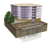
**Geothermal Heating and Cooling:** Geothermal energy originates from the heat retained within the Earth's core. Geothermal is a central heating and/or cooling system that pumps heat to or from the ground. It uses the earth as a heat source (in the winter) or a heat sink (in the summer). This design takes advantage of the moderate temperatures in the ground to boost efficiency and reduce the operational costs of heating and cooling systems.
