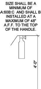
FIRE EXTINGUISHER CABINET
