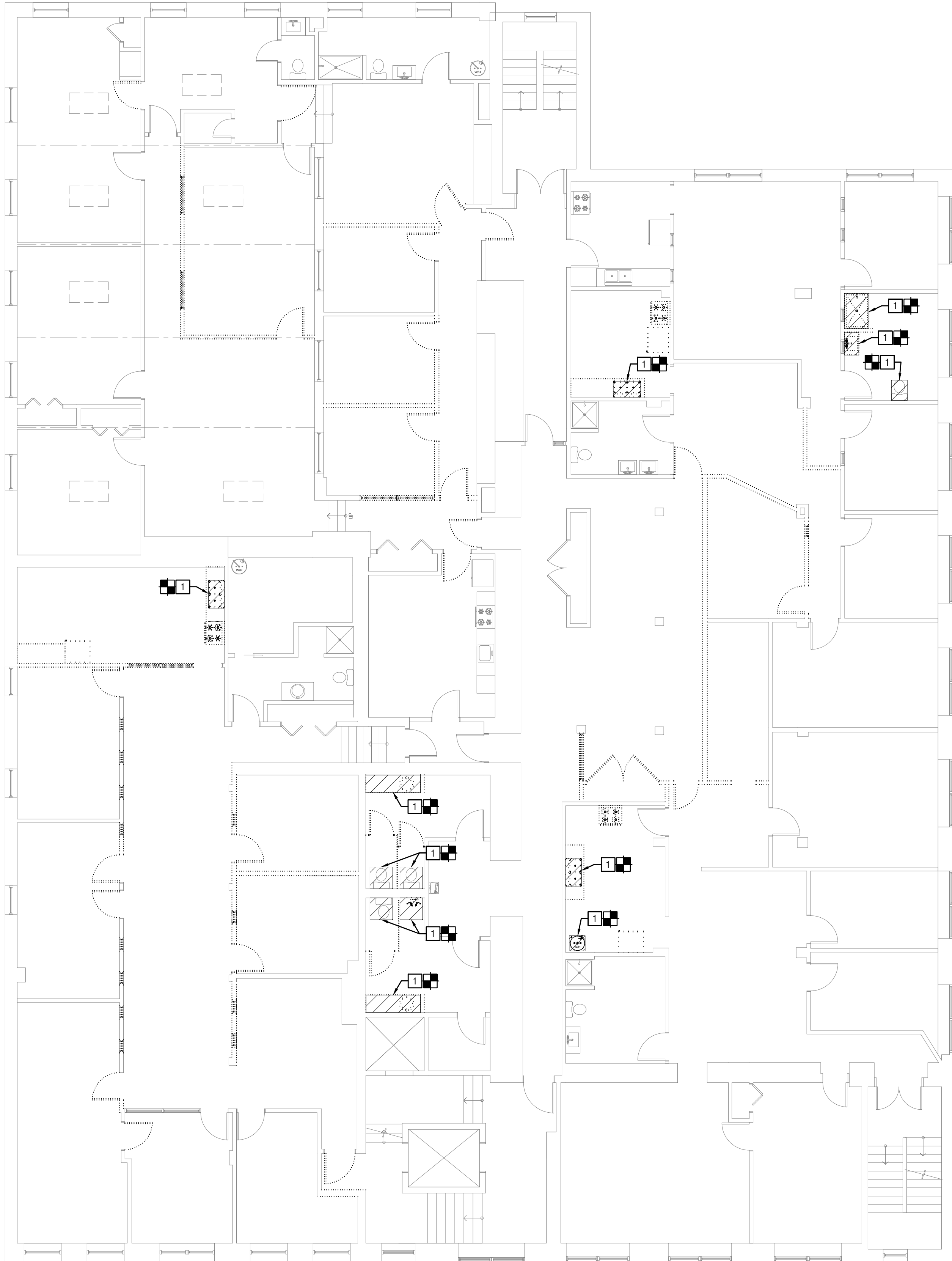
2 PLUMBING DEMOLITION PLAN - THIRD FLOOR P-3 SCALE: 1/8" = 1'-0"
