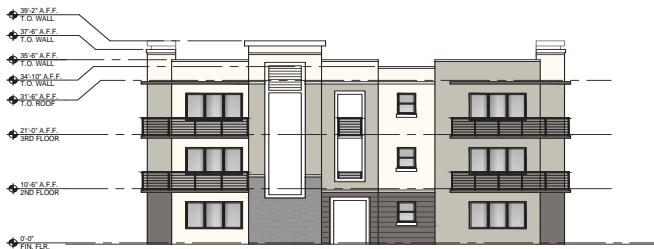
04 WEST ELEVATION BUILDINGS 1 & 2 SCALE: 3/32" = 1'-0"
