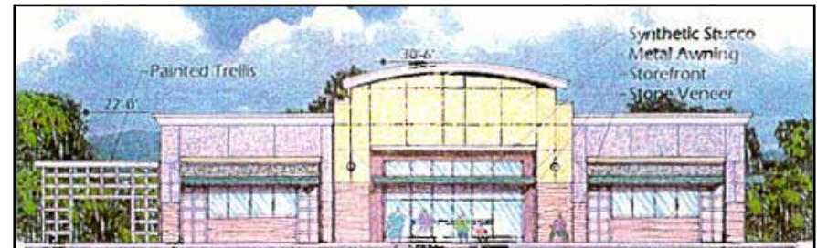
RESTAURANT BUILDING 'L' SOUTH ELEVATION
