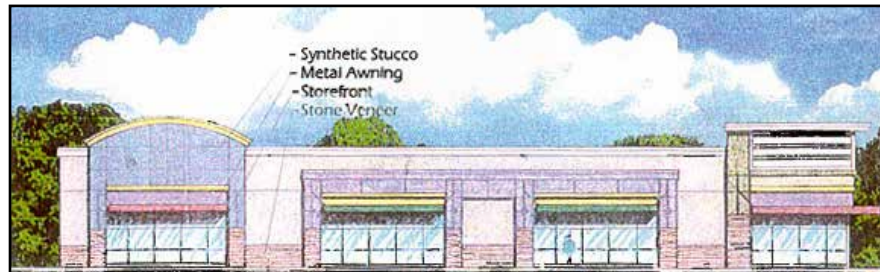
RETAIL BUILDING 'K' NORTH ELEVATION
