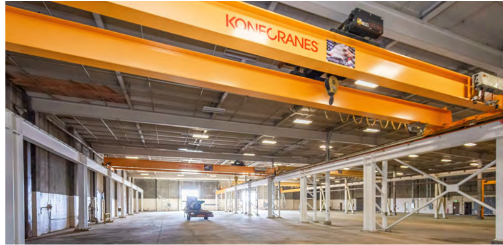
Unit A: Two (2) 10-Ton Top-Running Girder Bridge Cranes (Separate from Previously Pictured Cranes)
