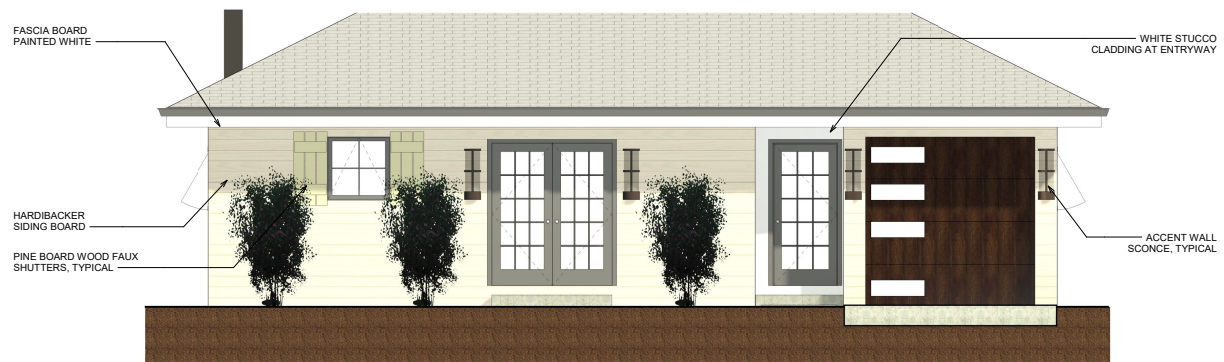
② UNIT B ARCHITECTURAL ELEVATION 3/8" = 1'-0"
