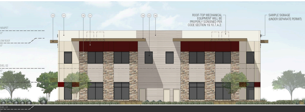
SOUTH WEST ELEVATION
