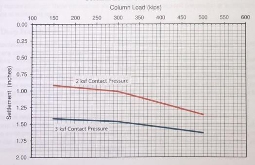
As shown on the figure, considering a tolerable settlement of 1 inch, column loads less than 300 kips can be supported on shallow spread footings designed using a net allowable bearing pressure of 2 ksf. Column loads greater than 300 kips will need to be supported on deep foundations and are discussed in subsequent sections.
