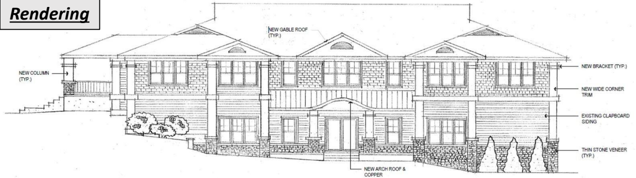
1 PROPOSED SOUTH ELEVATION - OPTION #2 SCALE: 1/8"=1'-0"
