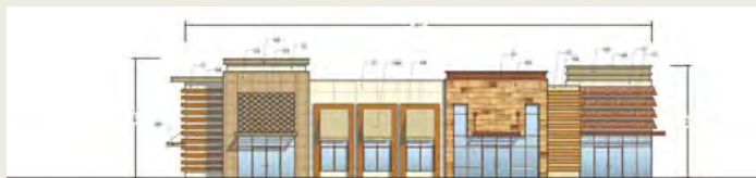
Building D3 West Elevation Scale 1/8"=1'-0"
