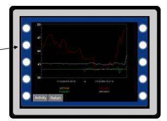
To select the different graph values, click one of the four radio buttons and then on the drop down. Select the desired parameter.
