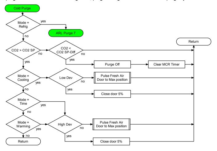
If the system is running in Cooling and the CO2 level exceeds the CO2 Setpoint, the fresh air doors will be pulsed open to the Max door setting. If during this opening of the fresh air doors, the plenum temperature drops below the Low Dev setting, the doors will be closed 5% until the plenum rises.
