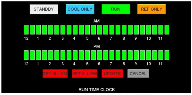
This screen shows the run time clock. To change click on the desired mode, STANDBY, COOL ONLY, RUN AND REF ONLY then click on the desired times. To save click on UPDATE. The SET ALL AM and SET ALL PM buttons can be used to set all the clock increments.
