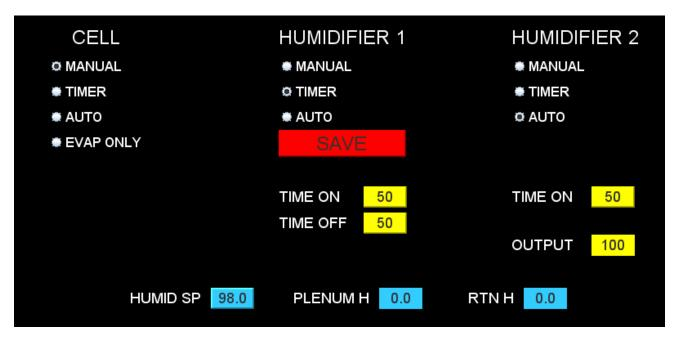
The Humidity screen allows all the humidity parameters to be set. See section 5.10 for more information.
