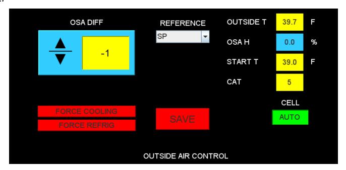
The OUTSIDE AIR CONTROL screen allows for the setting of the outside air differential and the reference. These values are used to calculate the START T. Any time the Outside air temp is less than the Start temp
