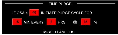
Four parameters must be set to initiate the time purge. In the above example if the outside air is less than 40 degrees initiate a purge cycle for 15 minutes every 6 hours and set the fans
