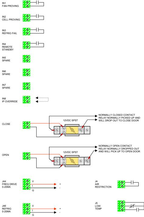
NOTE - LOW TEMP IS SHOWN IN NORMAL CONDITION. SHORT CIRCUIT MUST BE ON TOP TWO PINS FOR PANEL TO COME OUT OF SHUTDOWN.
