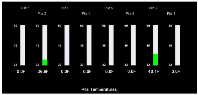
This screen shows the pile temps. The names of each of the pile sensors can be changed to reflect the location.
