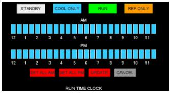
The warming mode is only used when trying to cure or warm up the product. During this time the time clock should be set to all blue and the Aux 2 switch should be set to Auto. Once the cure cycle is complete, the Aux 2 switch should be turned off.
