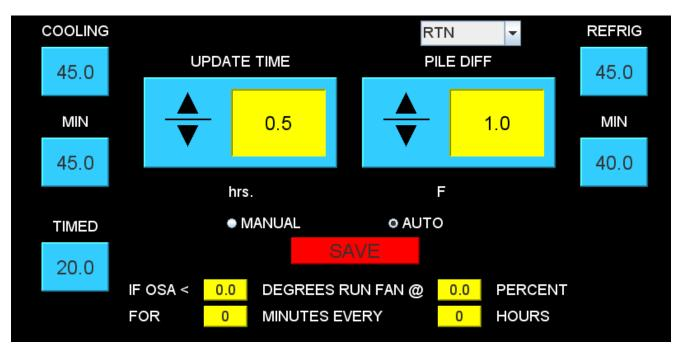
The Fan Speed Control page allows all setting for the speed of the Fan. See section 5.9 for more information.
