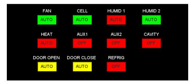
The Switch Status screen allow the user to view the status of all switches and remotely turn off or on. See section 5.12 for more information.
