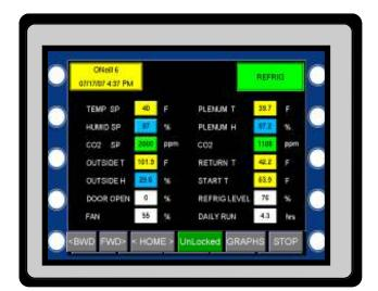
Pressing the GRAPH button from any screen will access the Graphing module
