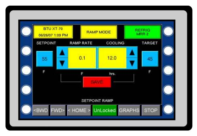
The SETPOINT RAMP screen allows the user to set up the ramp function. The ramp function will allow the setpoint to be automatically incremented to a target setpoint. An example of this could be seen in the fall. Once suberization has taken place, the ramp function could automatically drop the setpoint in small increments until the target temperature is reached.
