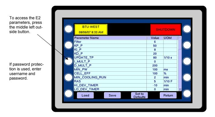
To change a parameter, press the value and a pop-up keypad will appear. Enter the desired number. Make multiple changes, if desired, and ,when done, press Save and then Return. If Set to Defaults is pressed, the default values for all parameters will appear. They are not saved until Save is pressed. Pressing the Load button will load the screen with the current values.
