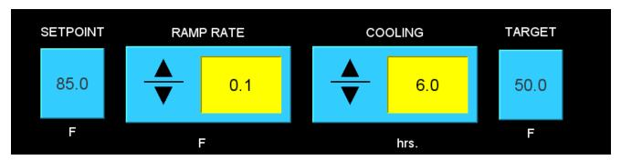
In this example, the Setpoint will be ramped down .1 degrees every 6 hours of Cooling. The ramp will shut off when the final Target temperature of 50 degrees is reached. Note - any-time the Setpoint is changed from the main screen, the Target will be reset to the Setpoint and the ramp will turned off.
