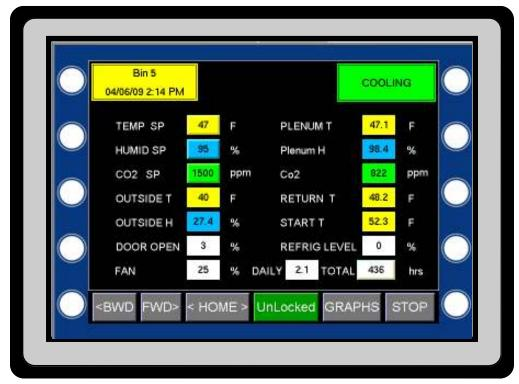
Note - to make any change to a system parameter, the Unlocked button must be green. See 5.3 on how to lock and unlock the system.
