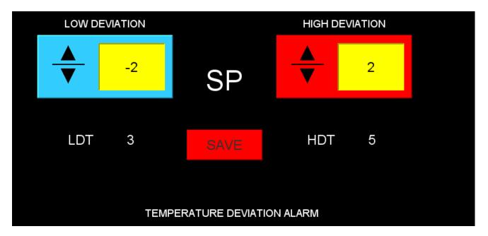
The Temperature Dev alarm screen allows the setting of the High and Low deviation. The LDT is the low deviation timer in minutes. It is a count down timer that is active when ever the plenum is below the setting. When the timer counts to zero it will trigger the alarm. The HDT is a similar timer for the High Deviation.
