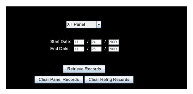
The Records button will allow the downloading of the records. The XT now stores two types of records, one for the XT panel and one set for the refrigeration system. Use the drop down to select the type of records first. Next enter the Start Date and End Date for the records. Click on the Retrieve Records button. A pop up screen should allow you to select Excel spread sheet for the download. See appendix for more information.
