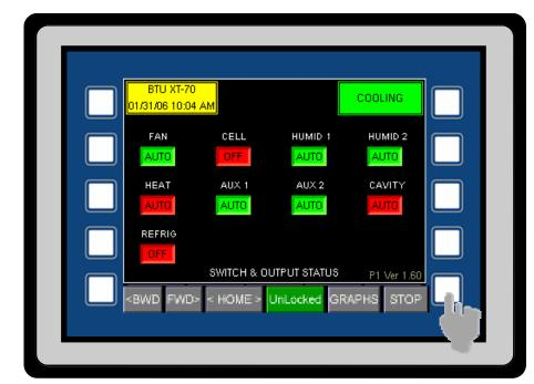
In order to place the XT panel into a test mode, first go to the SWITCH & OUTPUT STATUS screen. Once at this screen, press the bottom right outside button.
