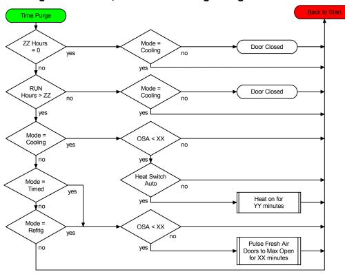
When the CO2 purge is triggered in the Cooling mode, it will be because the OSA is cold and the fresh air doors are only slightly cracked. The return air heaters will cause the air to warm by 3 to 4 degrees, causing the fresh air doors to open and the fans to speed up to purge the storage.
