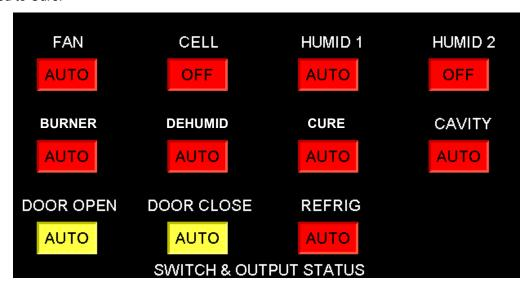
This shows the HMI layout, the actual switches on the panel need to be relabeled.
