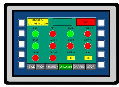
When the XT panels goes to the Test mode, all normal operation is suspended.
