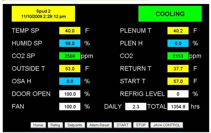
This screen is accessible using most cell phones and web browsers. The JAVA CONTROL button should only be used if you have a web browser that will run Java Applets. Most cell phones will not. If Java is not available then use the Refrig, Setpoints, Alarm Reset, START and STOP buttons.
