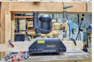
New PM2700 Shaper with more features than any other shaper in the same class. Extra large 30" x 40" precision ground cast iron table with heavy duty miter gauge and aluminum extruded support. Digital readout for spindle height allowing adjustments to within .001" in the spindle height (critical when aligning rail and stile cutters for raised panel doors).
