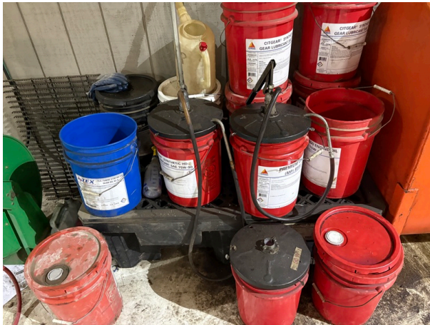
Five-gallon drums. Some stored on a spill pallet, others on the concrete ground surface.
