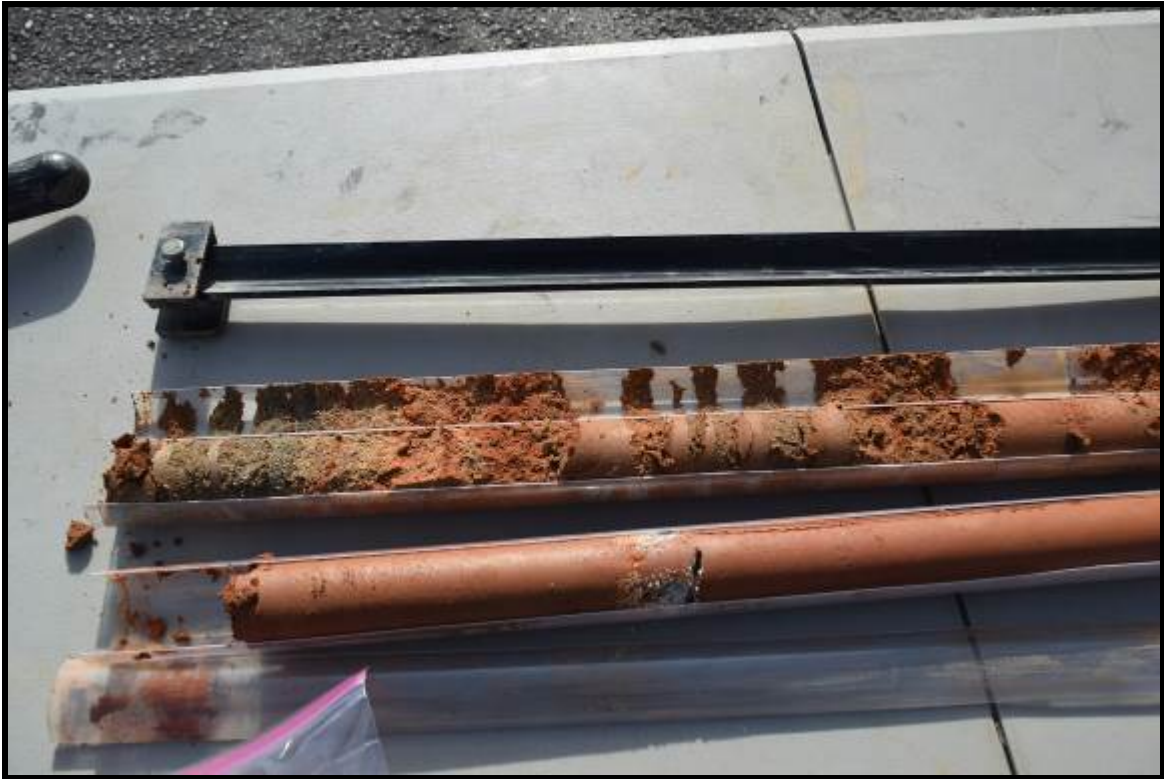
Photo 19: Typical soil cores collected during assessment of soils in the UST areas.
