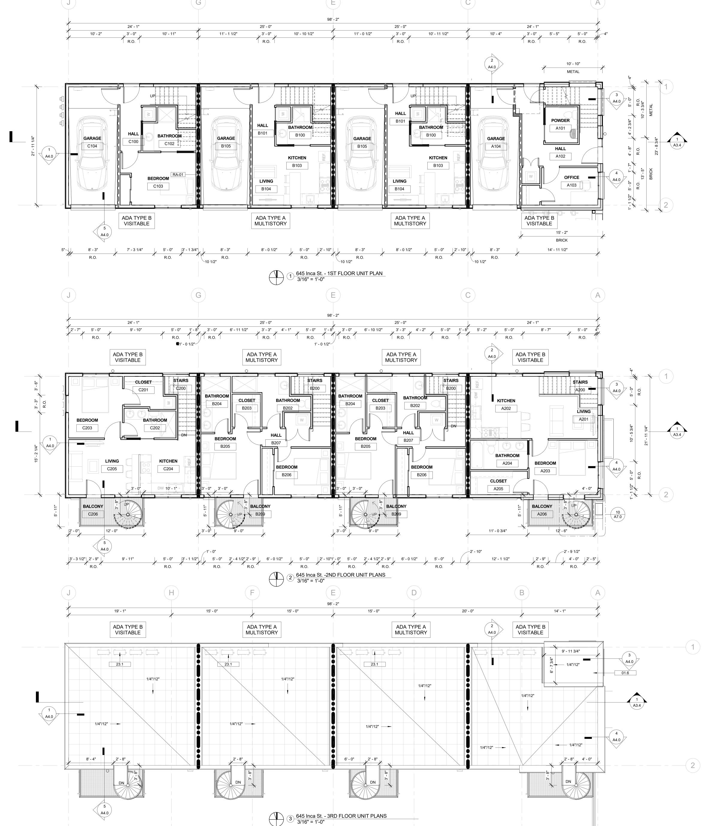
1. REFER TO OVERALL FLOOR PLANS (SHEETS A2.1-2.4 ) <u>ONLY</u> FOR ALL EXTERIOR FRAMING DIMENSIONS, WINDOW AND EXTERIOR DOOR CALLOUTS. GRIDLINES ARE TO EXTERIOR FACE OF FOUNDATION AND ALIGN WITH THE FACE OF STUD @ STUCCO AND PANEL SYSTEM AND WITH THE FACE OF BRICK @ BRICK SYSTEMS. EXTERIOR WALLS ON INTERIOR PLANS ARE FOR REFERENCE ONLY!
