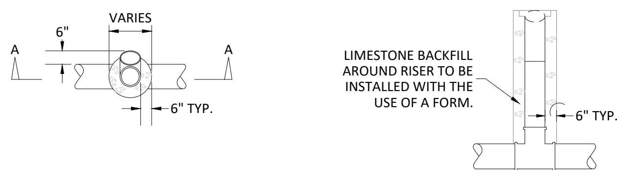
SEWER SERVICE CONNECTION (WITH RISER)
