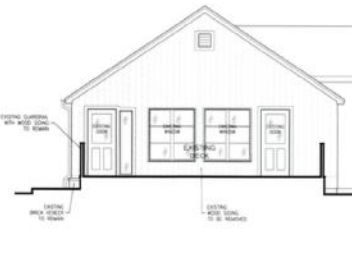
EAST EXTERIOR ELEVATION - DEMOLITION SCALE: 1/4" = 1'-0"
