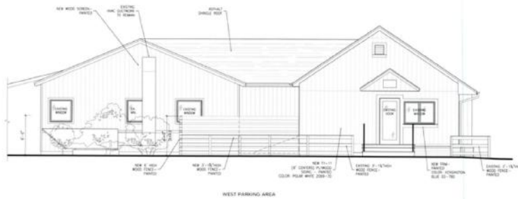
WEST EXTERIOR ELEVATION - PROPOSED SCALE: 1/4" = 1'-0"
