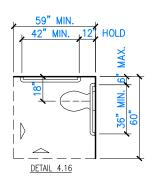
A. FOR WATER CLOSETS NOT LOCATED IN TOILET STALLS, THE FOLLOWING GRAB BARS SHALL BE PROVIDED, 33" - 36" ABOVE THE FINISH FLOOR:
