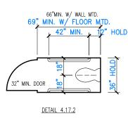
TAS SECTION 4.17.6 - GRAB BARS (REFERENCE DETAILS 4.16.2, 4.16.3, 4.17.1 & 4.17.2) A. GRAB BARS SHALL BE MOUNTED 33" - 36" ABOVE THE FLOOR. REFER TO 4.26 GRAB BARS FOR SIZE AND STRUCTURAL REQUIREMENTS.
