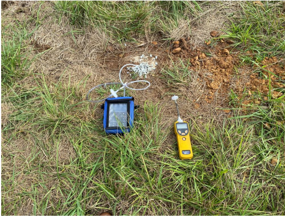
Photo 5 – Soil Gas Screening with GEM-5000 and PID
