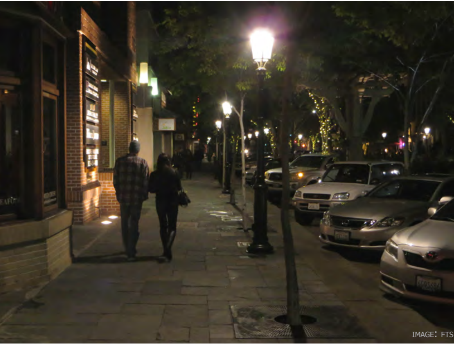
FIG. 3.1.5.G.1: EXAMPLE OF DECORATIVE PEDESTRIAN-HEIGHT POST-TOP LIGHTING SUPPORTIVE OF A SUCCESSFUL NIGHT-TIME WALKABLE COMMERCIAL DISTRICT SETTING - 12 FOOT HIGH POLES AT 50 - 70 FOOT SPACING WITH 100 WATT WARM WHITE (2700 DEGREES KELVIN) METAL HALIDE LAMPS (EQUIVALENT PERFORMANCE LED LIGHT SOURCES ARE ALTERNATIVES).
