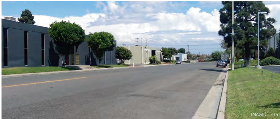
FIG. 3.1.5.E.1: VIEW EAST OF MISSING SIDEWALK SEGMENTS AT BOTH SIDES OF MT. WASHINGTON STREET BETWEEN EUCLID STREET AND TALBERT AVENUE
