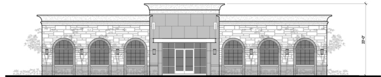
3 FRONT EXTERIOR ELEVATION PHASE 1 SCALE: 1/8"=1'-0"
