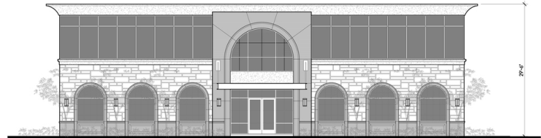
5 FRONT EXTERIOR ELEVATION PHASE 2 SCALE: 1/8"=1'-0"
