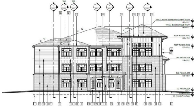
BUILDING 1 - RIGHT SIDE ELEVATION 4 SCALE: 3/32" = 1'-0" A3.0
