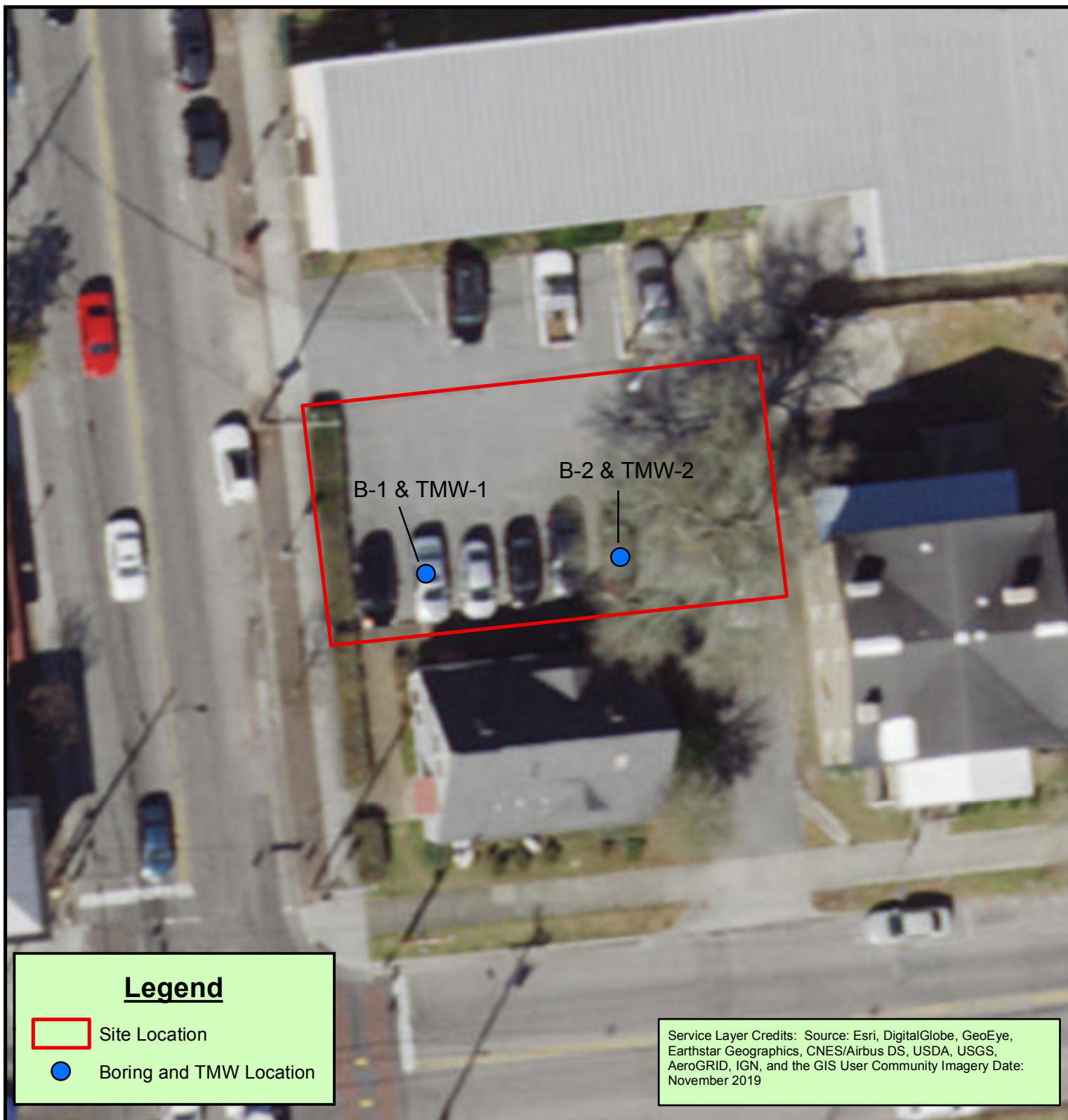
Figure 2: Boring and Temporary Monitoring Well Locations
