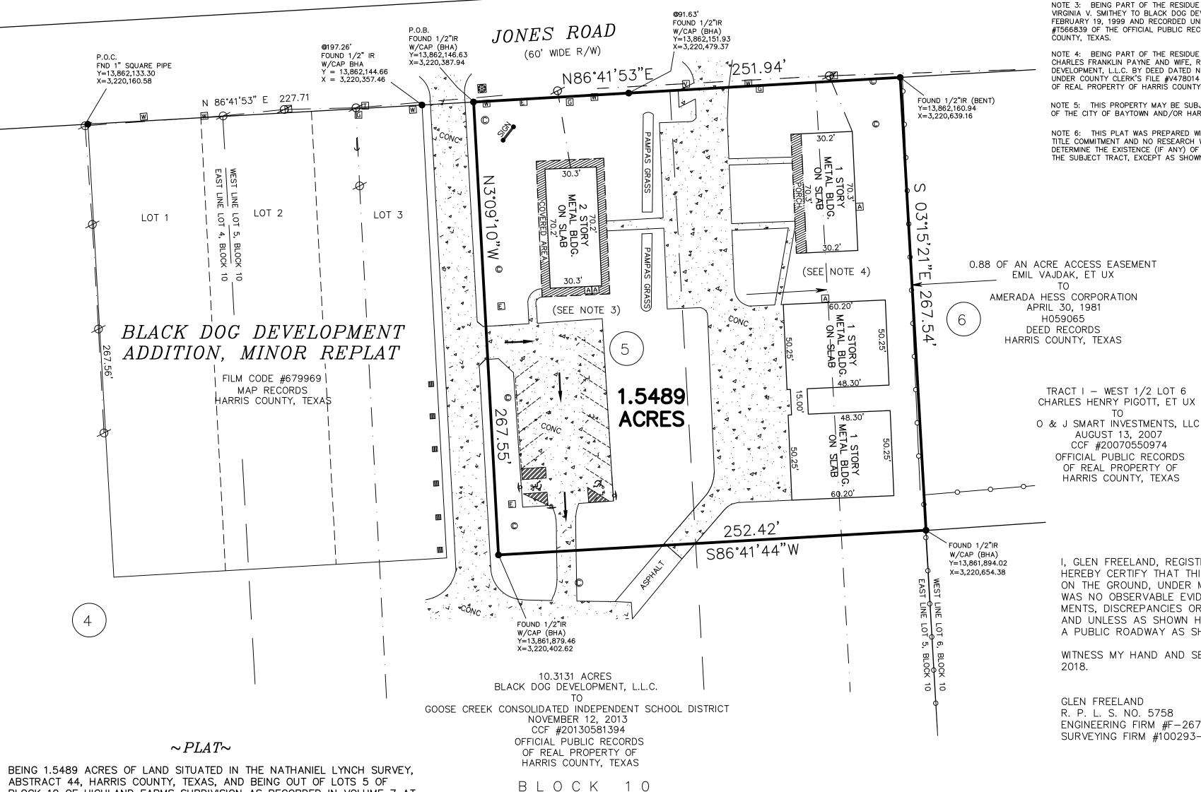
NOTE 1: BEARINGS ARE LAMBERT GRID BEARINGS AND ALL COORDINATES REFER TO THE TEXAS STATE PLANE COORDINATE SYSTEM, SOUTH CENTRAL ZONE, NAD 83. ALL DISTANCES ARE ACTUAL DISTANCES. SCALE FACTOR = 0.9997599. REFERENCE IS MADE TO THE METES AND BOUNDS DESCRIPTION OF EVEN DATE ACCOMPANYING THIS MAP.
