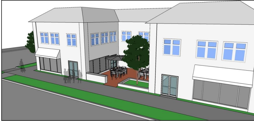
Figure 1327.F: An example of a forecourt used as dining space for a ground floor restaurant. Note that the forecourt is mostly enclosed except for on one side by the building.
