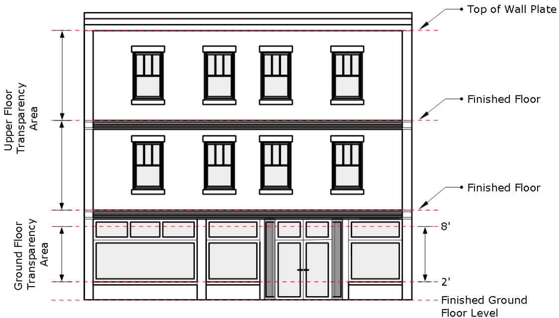
Figure 1315.J: Ground and Upper Floor Transparency Area
