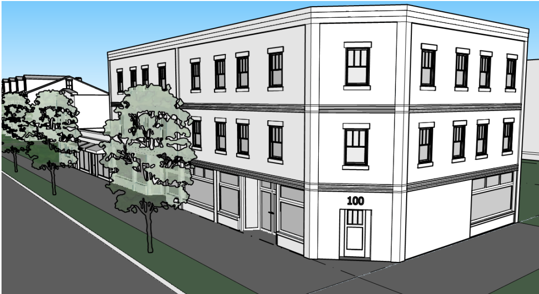
Figure 1315.D: Example of a chamfered corner
