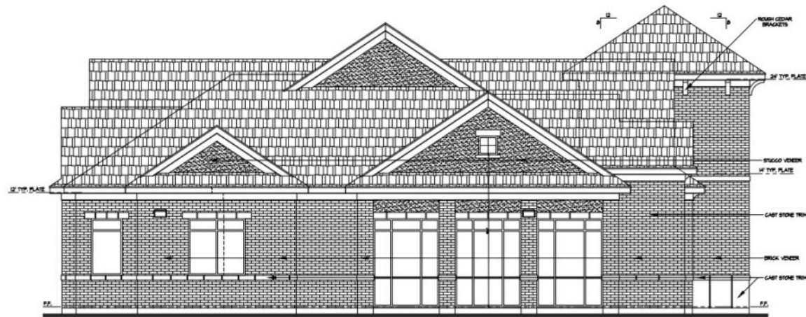
LEFT (SOUTH) ELEVATION SCALE: 1/4"=1'-0"
