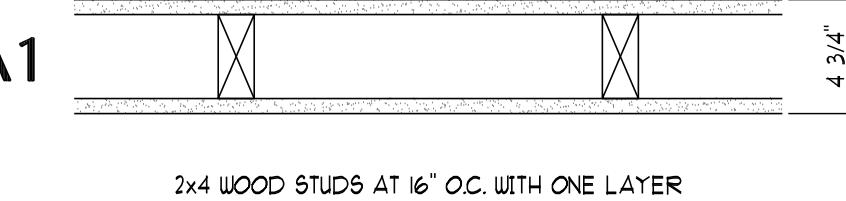
2x4 WOOD STUDS AT 16" O.C. WITH ONE LAYER
