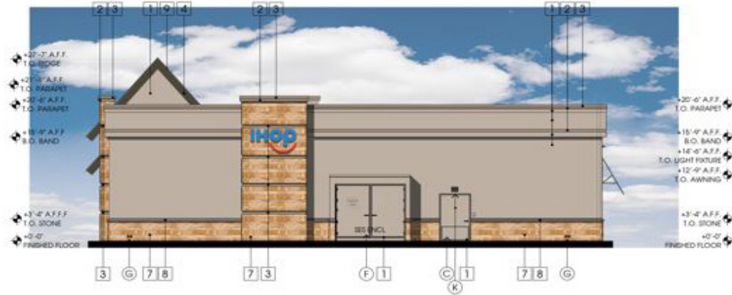
B ELEVATION (WEST) FACING ENTRY DRIVE SCALE: 1/8" = 1'-0"
