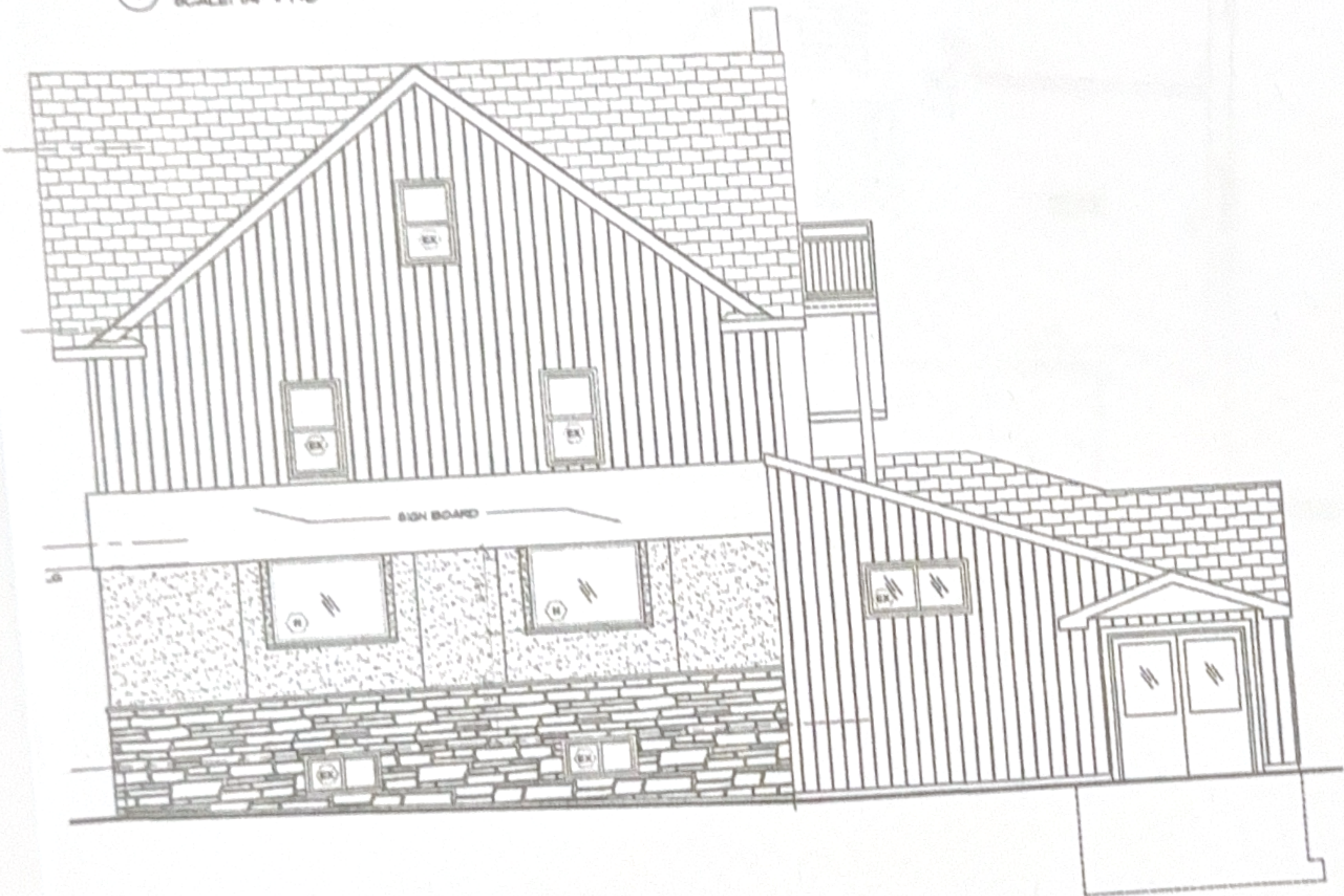
2 NORTH SIDE ELEVATION SCALE: 1/4" = 1'-0"
