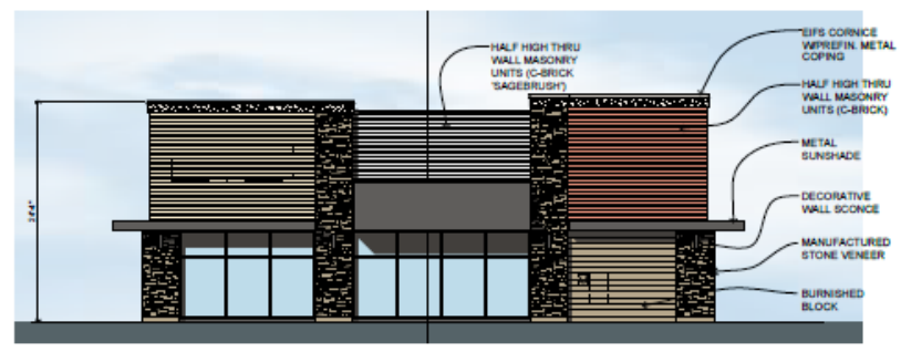
Bldg. A - East Elevation 1/8" = 1'-0"
