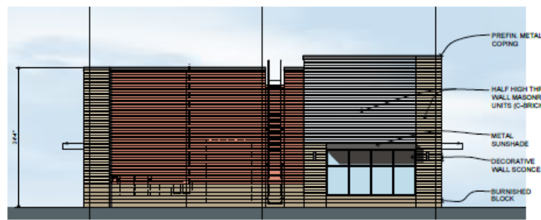
Bldg. A - West Elevation 1/8" = 1'-0"
