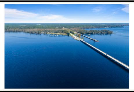
New First Coast Expressway bridge under construction over the St. Johns River just south of where the Shands Bridge stands currently. The vertical height clearance of the new bridge will be 65 feet. The additional 20 feet of clearance will match the Buckman Bridge's clearance to the north removing all barriers for marine traffic.
