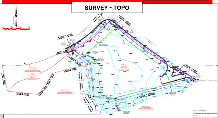
Bearings shown hereon are based on the East Line of the Northeast 1/4 of Section 25, Township 22 S, Range 31 E, as being S 00°13' 56" E per state plane coordinates Florida East Zone, per reference points CCR # 106075 & CCR # 77286.
