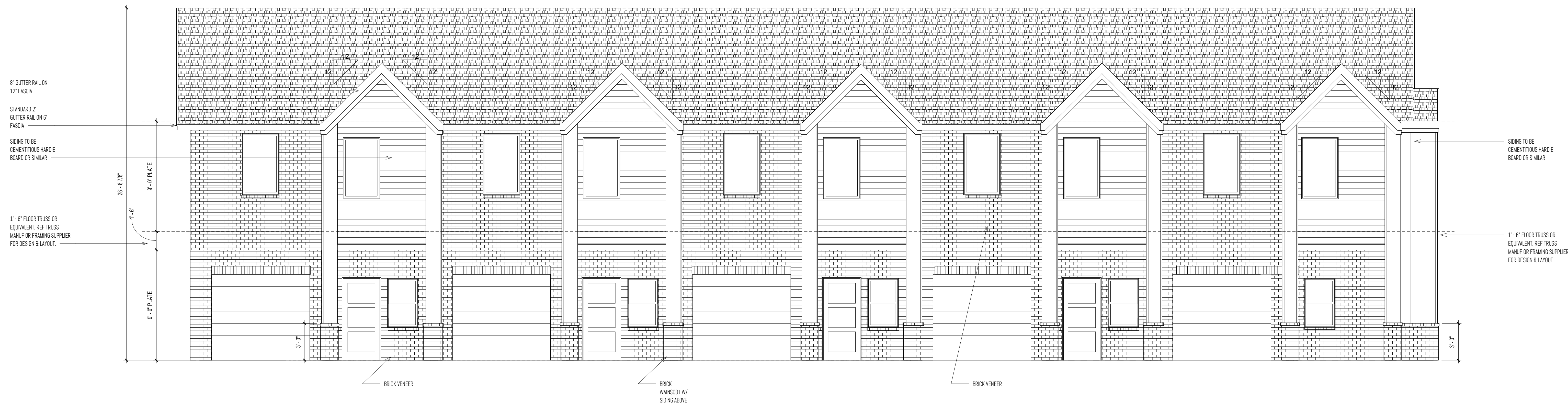
① FRONT ELEVATION 1/4" = 1'-0"
