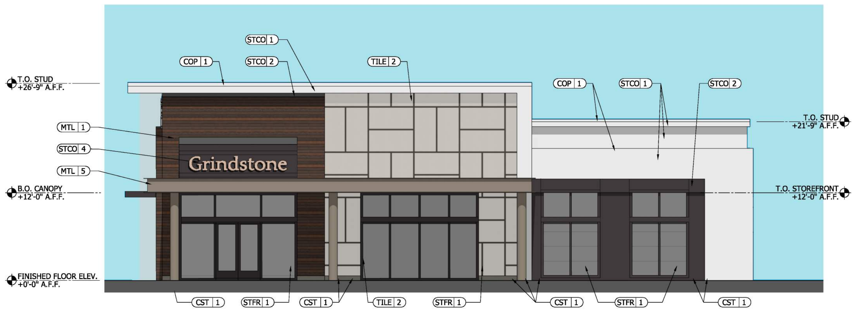
4 A301 BUILDING D WEST ELEVATION SCALE: 1/8" = 1'-0"
