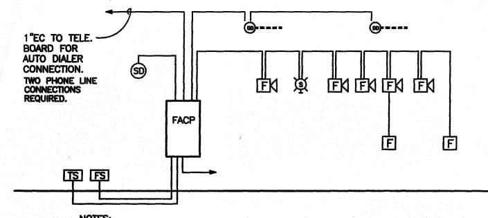
1. FACP SHALL HAVE A MINIMUM 24HR. BATTERY BACKUP. 2. FACP SHALL BE FULLY ANALOG ADDRESSIBLE.
