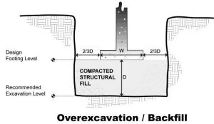
NOTE: Excavations in sketches shown vertical for convenience. Excavations should be sloped as necessary for safety.
