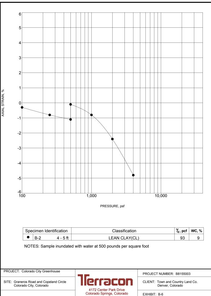
SWELL CONSOLIDATION TEST ASTM D4546
