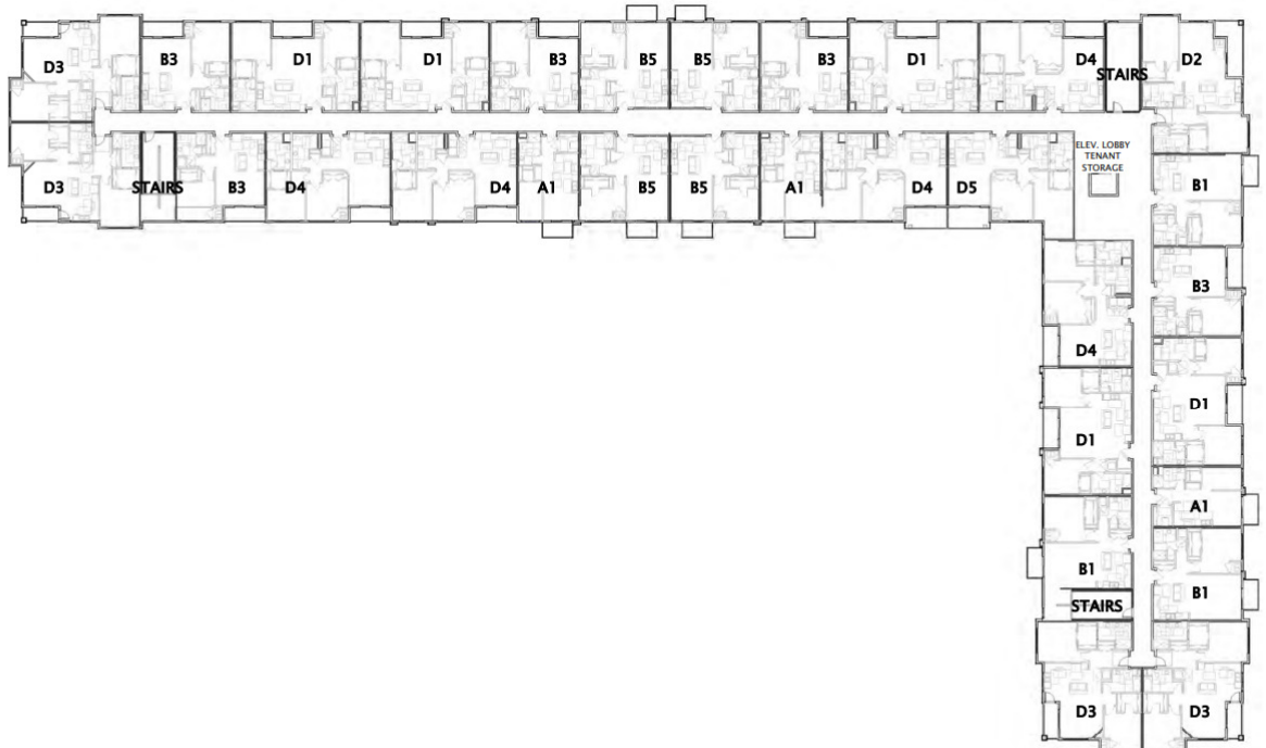
① CONCEPTUAL FOURTH FLOOR PLAN 1" = 30'-0"
