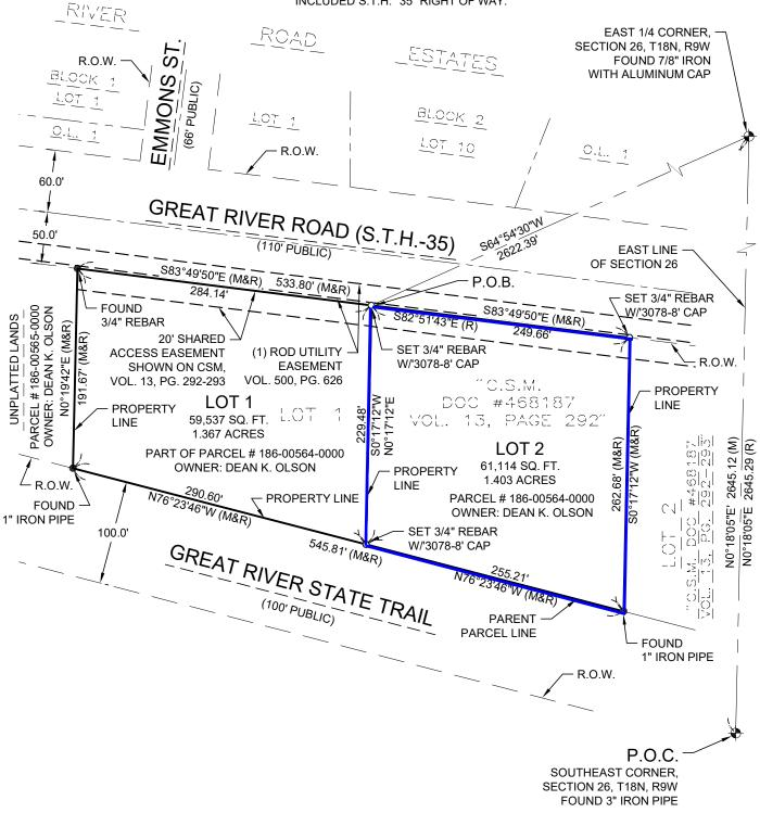
The basis for bearings is: BEARINGS ARE REFERENCED TO THE WISCONSIN COUNTY COORDINATE SYSTEM, TREMPEALEAU COUNTY ZONE, NAD 83 (1991), ALONG THE EAST LINE OF SECTION 26 FROM THE SOUTHEAST CORNER TO THE EAST 1/4 CORNER, SECTION 26, TOWN 18 NORTH, RANGE 9 WEST, MEASURED AS N00°18'05"E.
