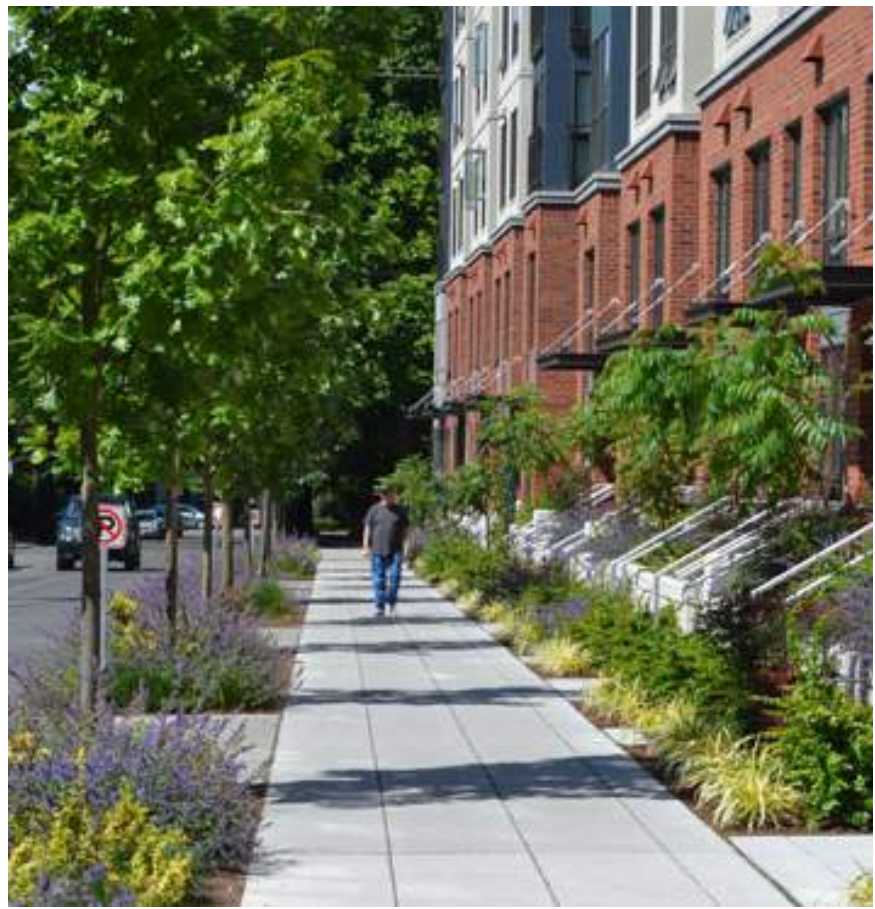
Frequent breaks in the parkway landscaping allow for more convenient pedestrian access to the street.
