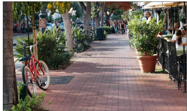
Example of an urban sidewalk, with landscape, pedestrian, and dining zones clearly delineated.
