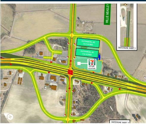
The proposed Kinston Bypass would be a four-lane, median divided freeway (accessible via ramps at interchanges) that extends approximately 21 miles from U.S. 70 near La Grange (in Lenoir County) to U.S. 70 near Dover (on the Jones-Craven county line). The project has a design speed of 70 mph and, when complete, would help reduce traffic congestion and delays that currently exist along U.S. 70 in Lenoir, Jones and Craven County.
