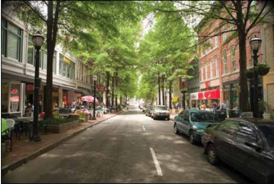
Figure 5.13. Roads are an important part of mixed use developments. This development along 15th Street in Atlanta, Georgia, has narrower roads to provide room for wider sidewalks that improve walkability.
