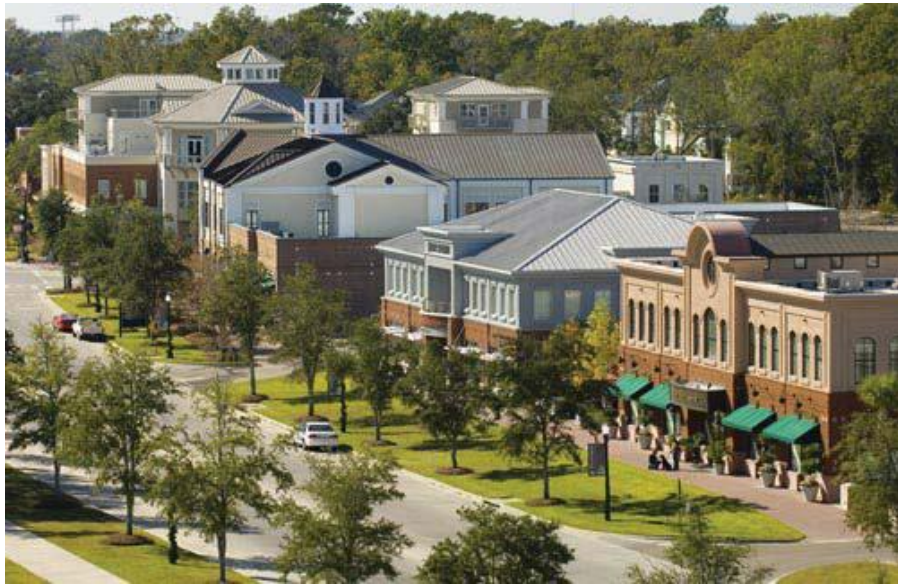
Desirable Design Attribute - buildings are placed along a “build-to” line with landscape buffer which creates a consistent and strong street wall along the corridor.
